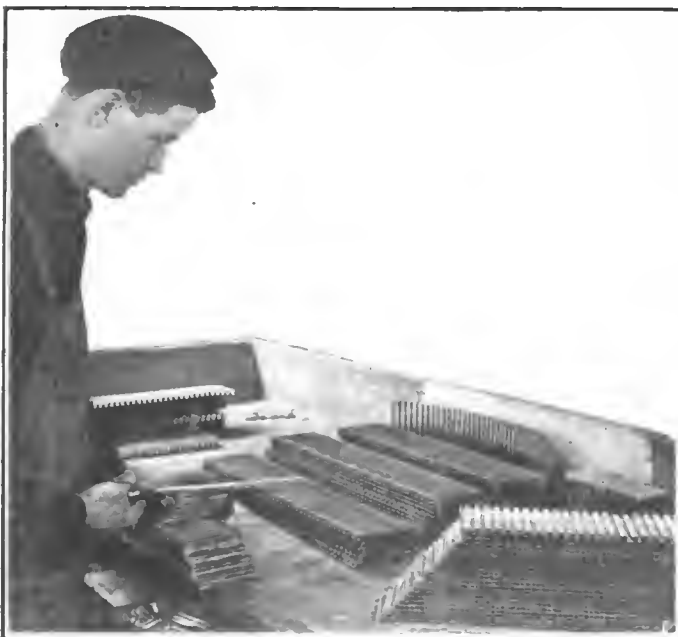
Stage 4—Cutting the tubes to conform to shape of frame
